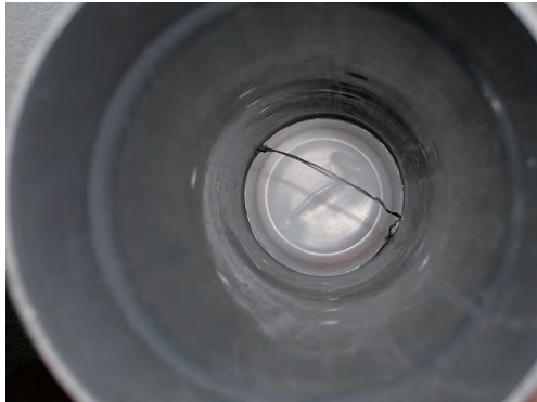
Fig. 12. Top view of component B placed in the bottom of component A of a MSS trap with handle up in pulling position (© MNCN; photographer: Miguel A. Alonso-Zarazaga).
