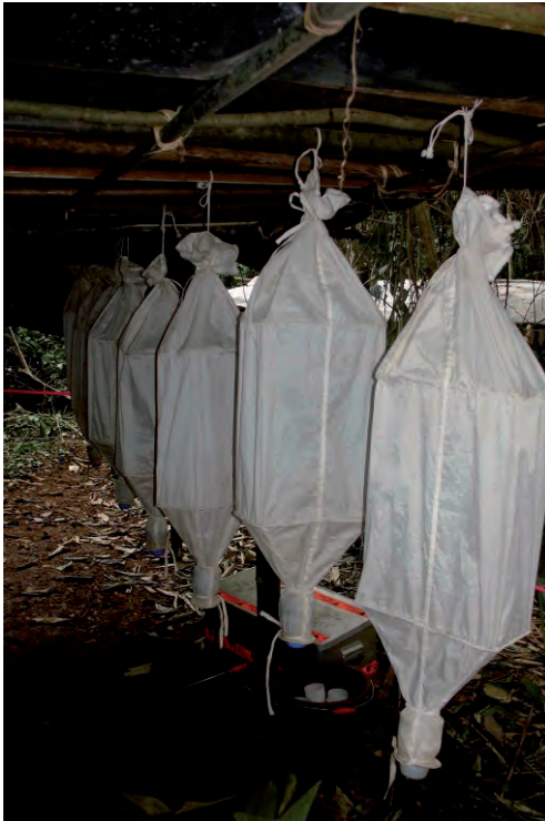
Fig. 15. Array of MoczarSKI electors in place at a field station in Mont Nimba (Guinea). (© and photographer: Didier VandenSpiegel).
